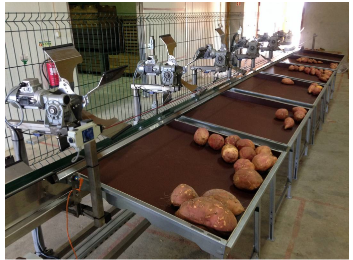
Exemple of a layout of a checkweigher with 6 outputs :
