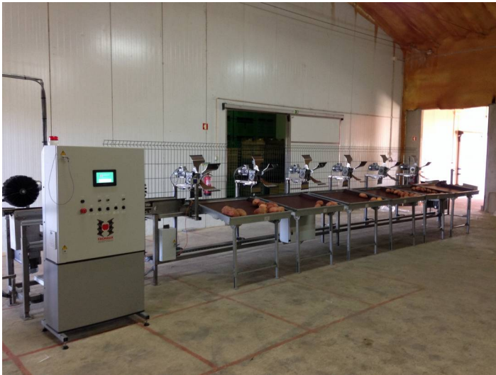
Exemple of a layout of a checkweigher with 6 outputs :
